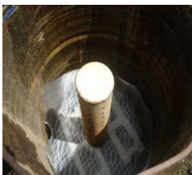
Set steel mesh on blocks – with a modified steel pipe on top of the mesh. The steel pipe needs to be sealed at the top with holes made on the side. This is to allow the steam from the boiling water circulate through your seed raising mix (photo PIFON).
