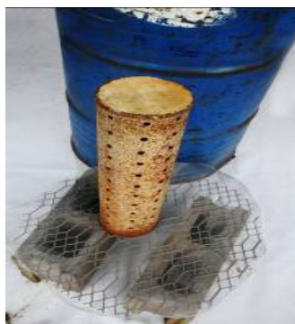
Place two (2) blocks at the bottom of a drum (photo PIFON)
