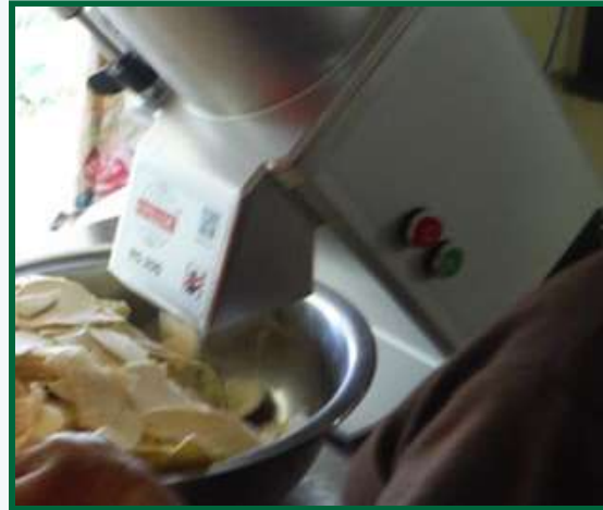
Figure 2b: A mechanized electric chip slicing machine used at the Tutu Rural Training Centre
