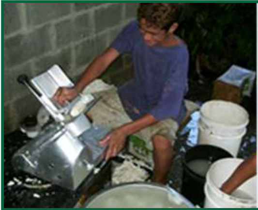
Figure 2a: Hand operated slicer in a village-based chip making enterprise in Samoa
