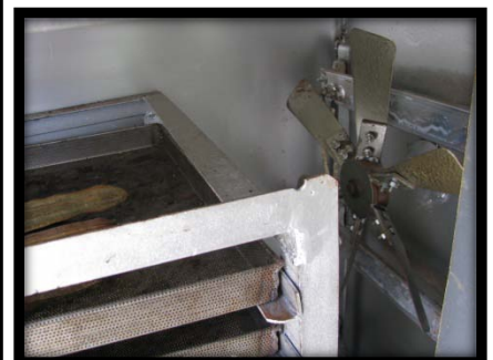
Picture 2 Inside view of electric generated drier (tray and fan) at National Exports Ltd- Lautoka
