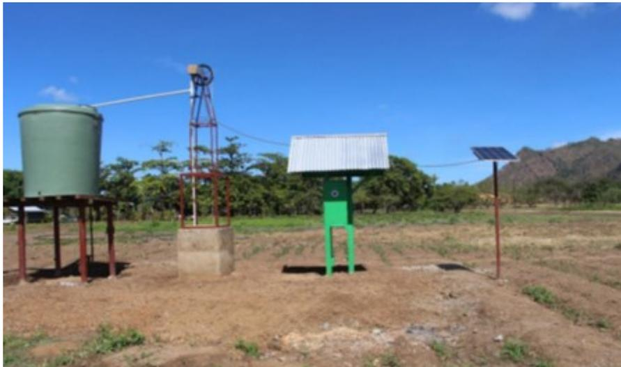
**Solar Powered Rope and Washer Pump Technology Demonstration**
