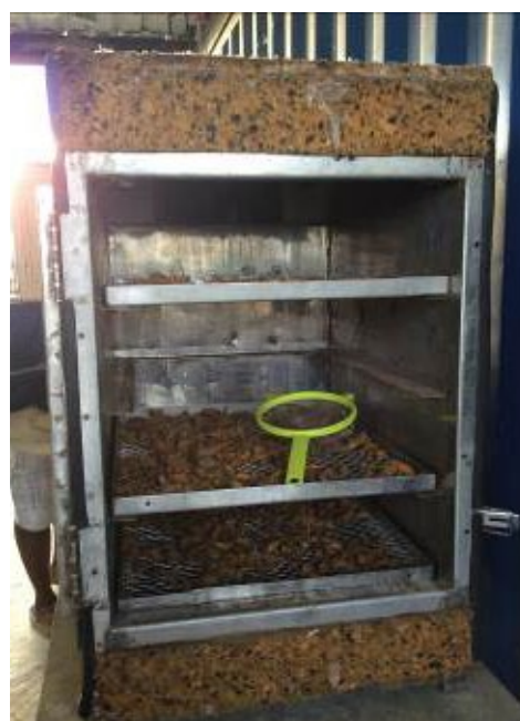
A hot air dryer used to dry breadfruit chips at Bula Agro Enterprises, Votualevu, Nadi, Fiji
