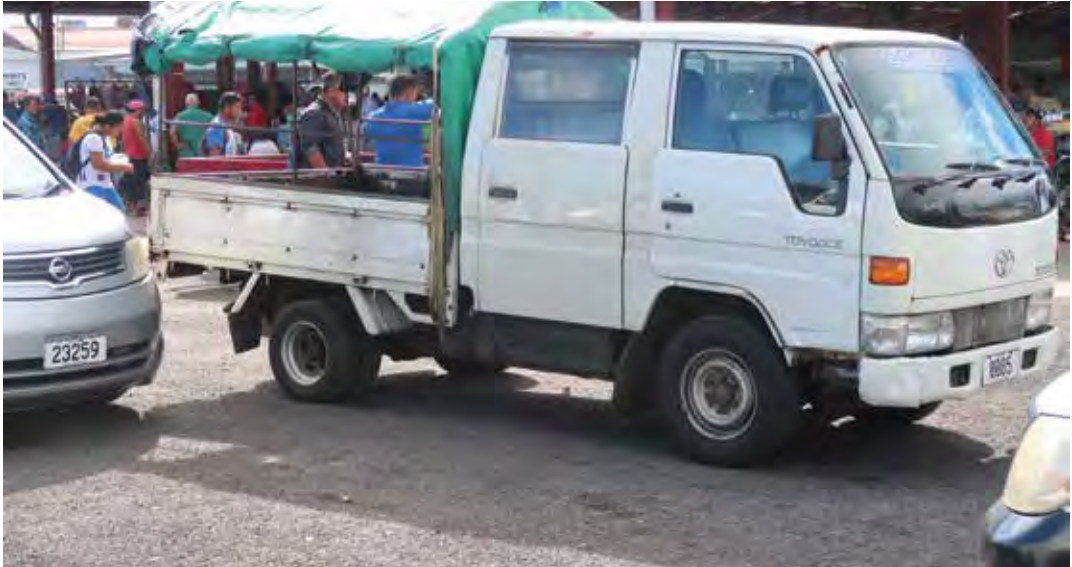
Photograph above: This is good truck setup. The tray back has a canvas covering, with roll-up sides, so produce is protected during transport and to make unloading easier.
