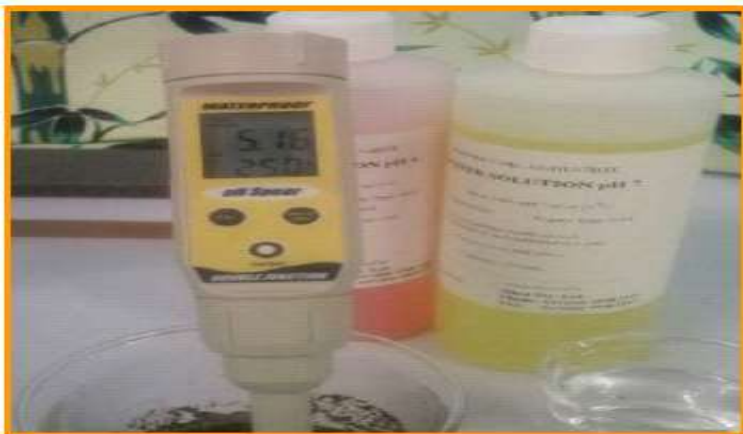
pH and moisture testing—cocoa pH testing falls between 4.5—5.5, moisture test-
