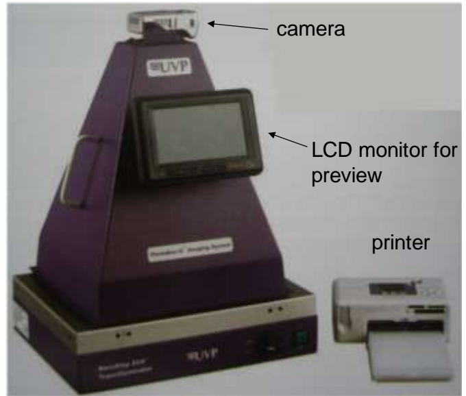
Transilluminator, with set up for viewing and photographing the gel.
