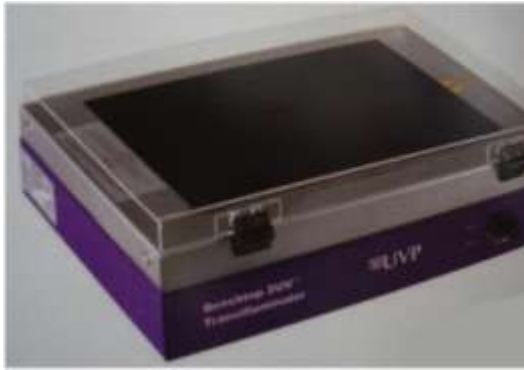
Transilluminator, with set up for viewing and photographing the gel.
